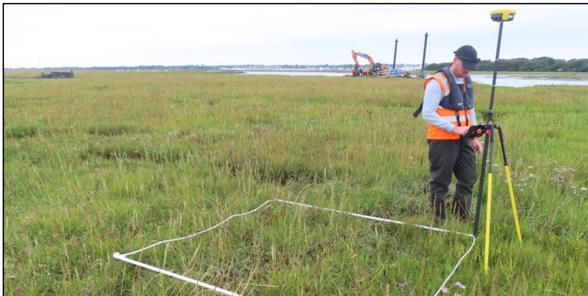
Image 4. Position and elevation recording of corners at quadrat Site Q4
