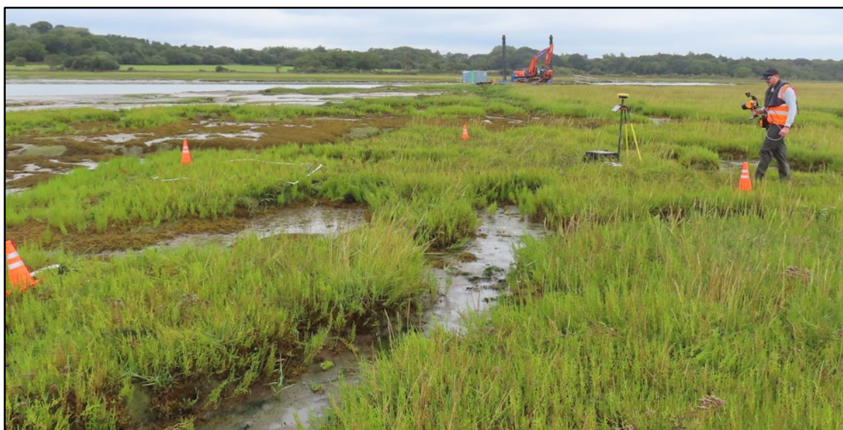
Image 5. GeoSLAM 3D LiDAR topography and photogrammetry mapping at Site Q3
